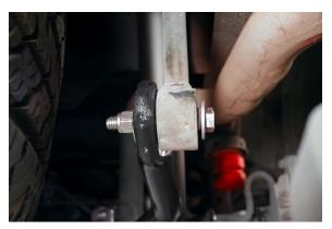
15. Adjust the position of the sway bar so it is vertically behind the axle. Torque the pivot bushing U-bolts to 44 ft lbs.
