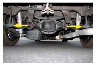
8. Remove the four 18mm U-bolt nuts at the axle clamp to detach the clamps and sway bar assembly from the vehicle.
