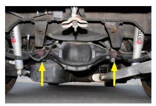
9. Remove the retaining clips from U-bolts holding the axle clamp on the axle and remove axle clamp assembly from the vehicle.
